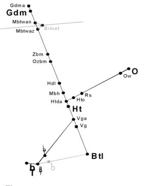
The main conflict area's are at Vught Aansluiting (Vga) and at Diezebrug Aansluiting (Htda) and also in 's-Hertogenbosch (Ht) itself. Additionally, headway conflicts frequently occur on the open tracks (e.g. between intercities and stopping trains or freight trains).
